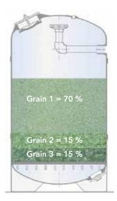
Grain 2 can be used for filters less than 1000 mm in diameter instead of grain 3. Also for all DIN filters with nozzle plate, grain 3 can be substituted with grain 2.
