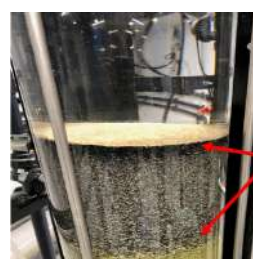
AFM® + Anthracite Depth & Surface Filtration
