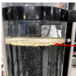
AFM® + Anthracite Surface Filtration
