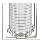
Open air purifier's rear cap, slide filter holder to the left to unlock and remove filter cartridge.
